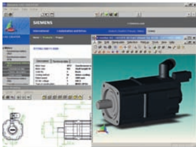
The CAD CREATOR provides a range of dimension drawings for the mechanical design
