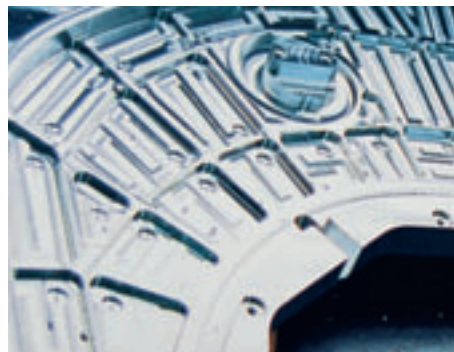
Five-axis machining of complex milled part
