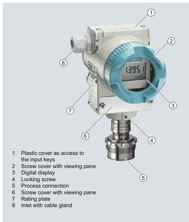
Device front view, SITRANS P DS III
