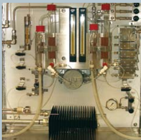
Siemens HRVOC water sparging vessel
